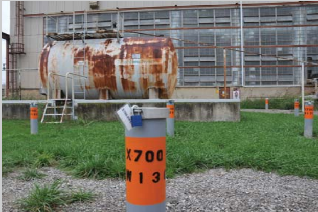
Groundwater monitoring wells located outside the X-700 former decontamination facility
